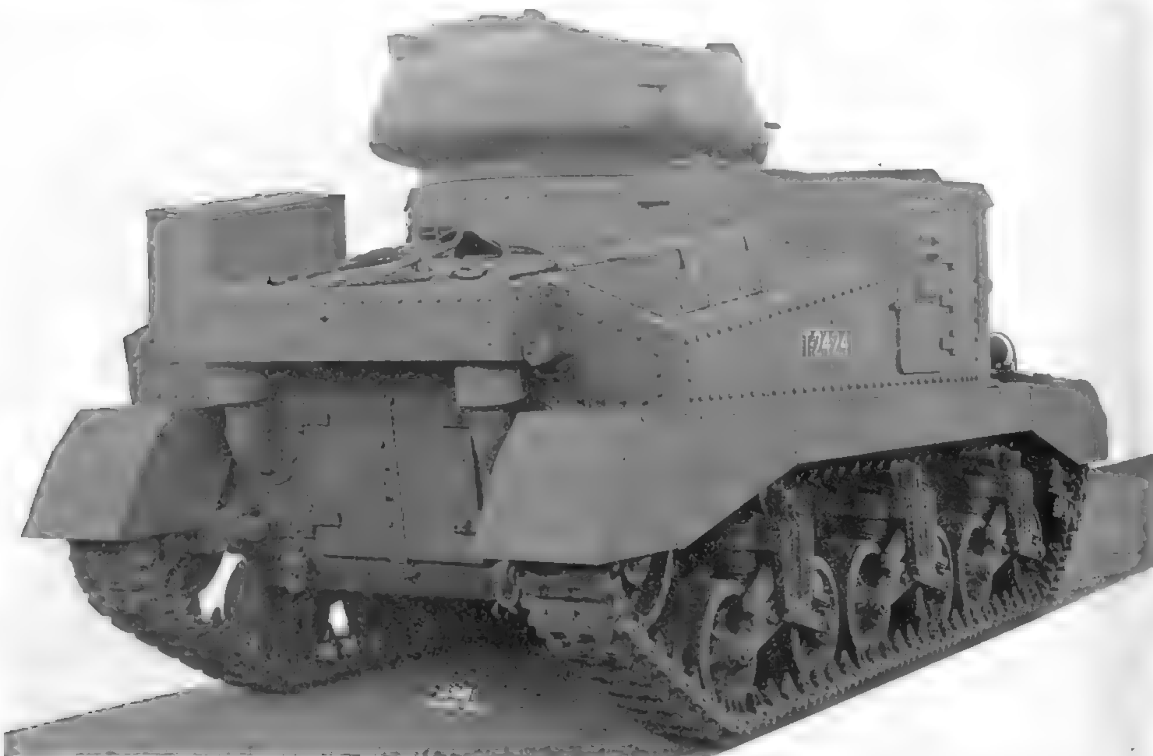
The British version of the M3 medium tank was the Grant. The two versions differed in turret shape and stowage boxes mounted on the rear deck. (National Archives and Records Administration photo)
